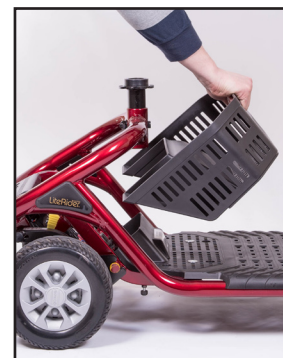
Remove the baskets from under the seat and from the tiller (not shown)
