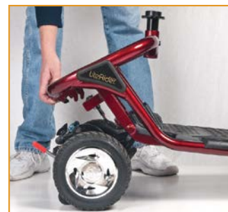
While squeezing the release lever, pull up on the rear frame
