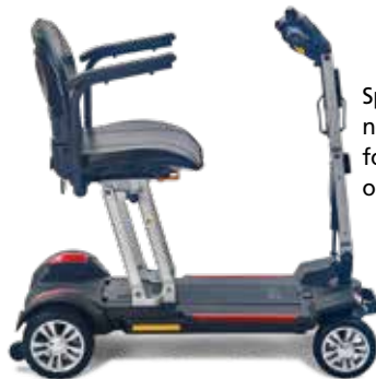
Tiller & self-locking seat frame fold for a compact profile
