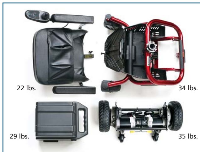
3. Grasp the frame and locking handle; lift the handle to unlock, and lift the frame up and off the drive train.
