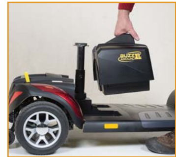
Step 2: Pull out the battery pack!
