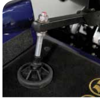
Hold-Tite foot securement for scooters (ASL-250A).
